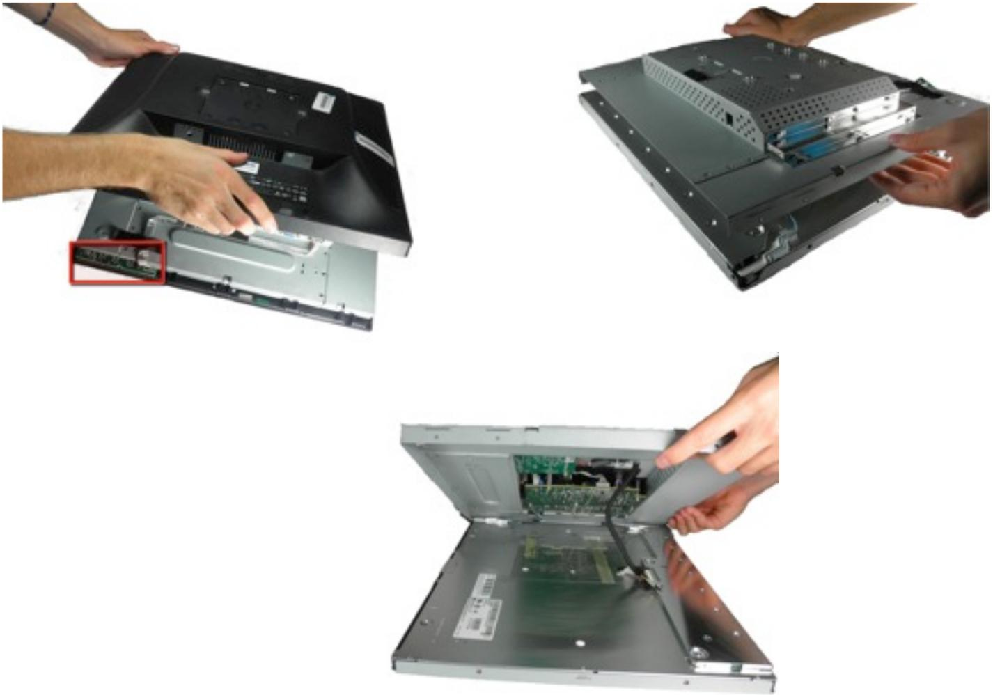
**Figure 12.** Deconstruction of an LCD monitor showing the back cover, printed circuit board mounting frame to which the printed circuit boards attach, and lightbox assembly (LCD screen package). Taken from: [http://www.ifixit.com/Device/Dell\\_E193FPc](http://www.ifixit.com/Device/Dell_E193FPc)
