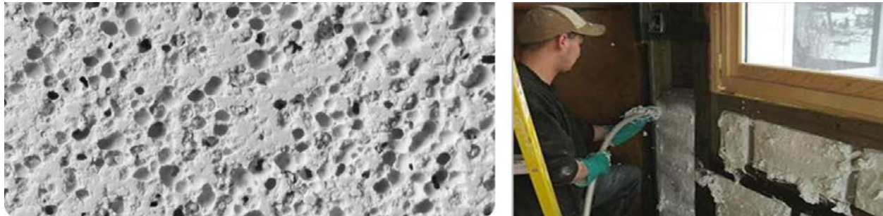
Figure 6. Foamed concrete material in close-up, and being applied.
